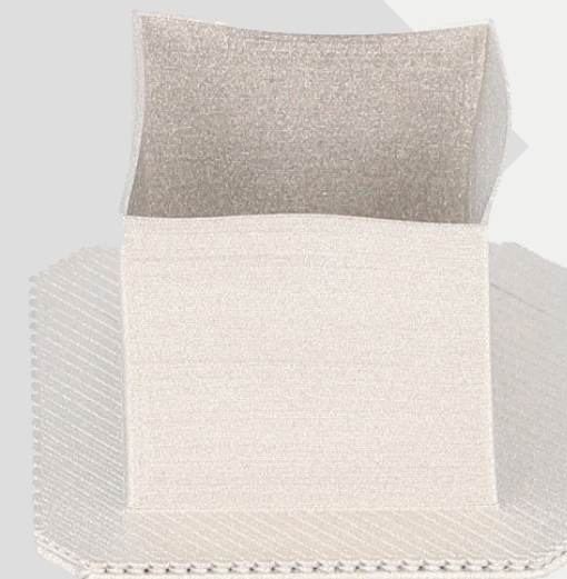
Figure 18: 0.4mm Wall Failure
