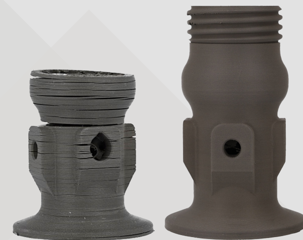
Figure 22: Cooling & Delamination Example
