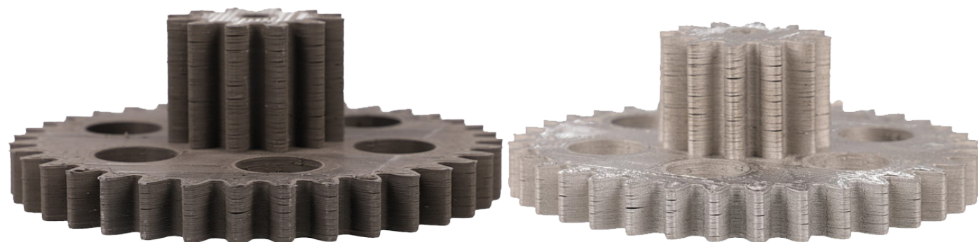
Figure 6: Print Delamination Become Sintered Cracks
