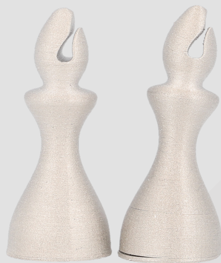
Figure 14: Warped Bottom Can Lead to Failure
