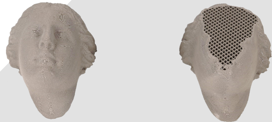
Figure 21: Mass Reduction Using Infill
